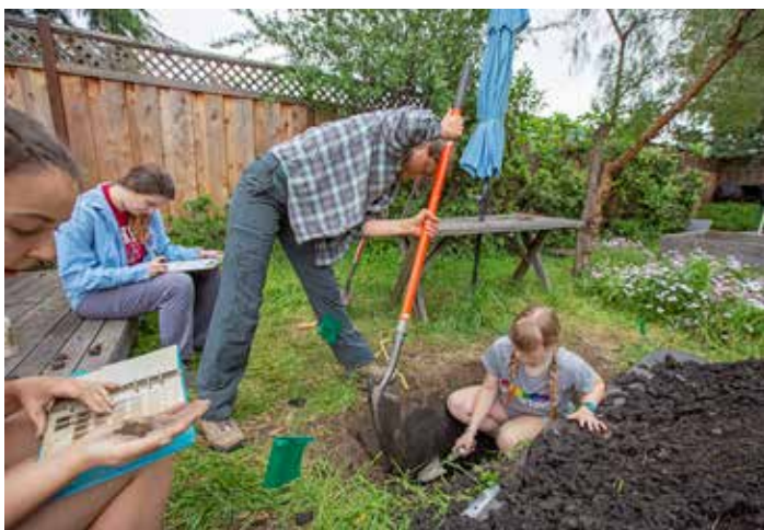
Students in the Cardinal Course Science of Soils dig a soil pit at the Green Beginnings Garden to classify the soils found at different depths, analyze soil texture, and collect soil samples for testing in the lab. Photo: Christine Baker.
